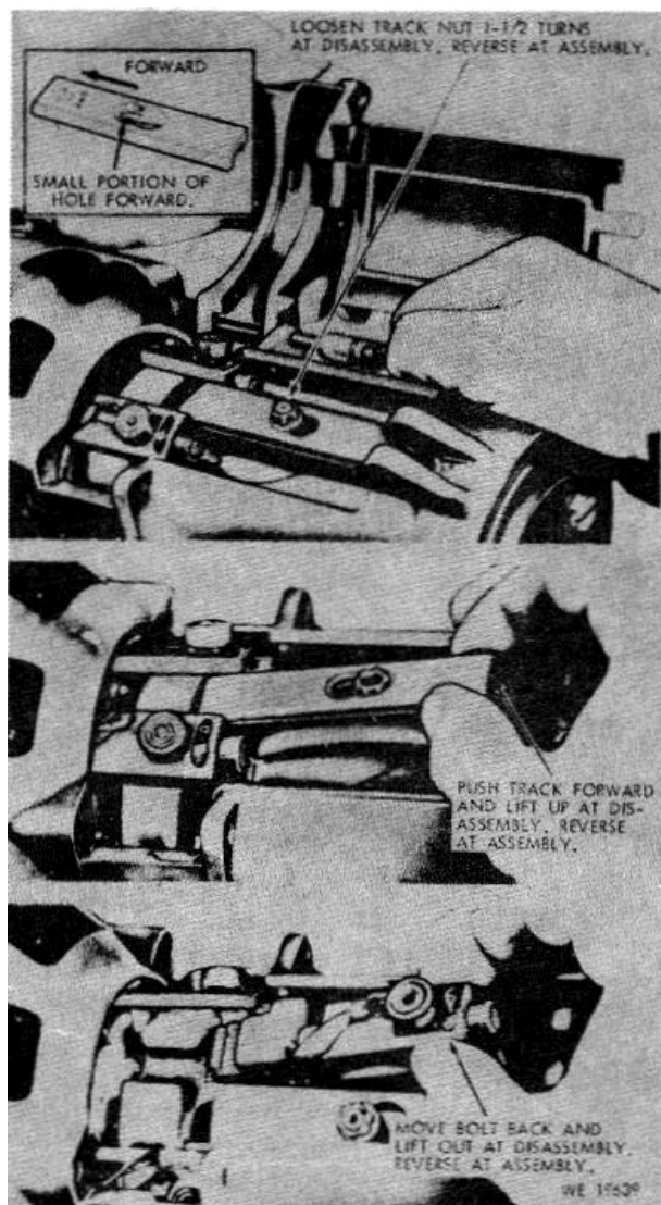
Figure 3-6. Installation/removal of track bolt assembly.
